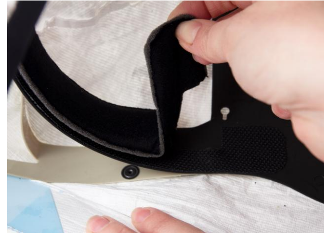
4.3 The sweat band is secured with Velcro tape to the forehead band. Pull the sweat band off.
