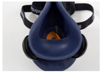
**1.3** Cut the tube so it does not touch the test persons mouth/lips.
