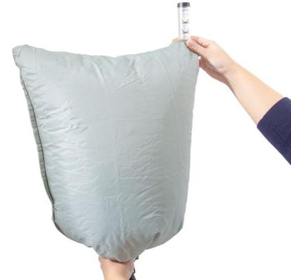
**2.3** Place the head top in the flow meter bag and start the fan unit.
