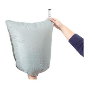
2.2 Place the head-top in the flow meter and start the fan unit. Grip the bag to seal around the breathing hose.Grip the flow meter tube with the other hand, the tube will point upwards from the bag
