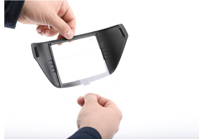
3.3 Fit a new protective lens.
