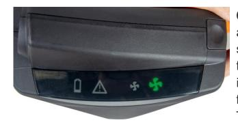
**6.4** If the button is pressed again, boosted operating status will be activated, with a flow at least 225 l/min. This is indicated by the larger green fan symbol lighting up. To revert to normal operation, press the control button once again.
