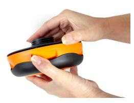
**10.1** Change particle filter by bending the pre-filter holder from the filter adapter.
