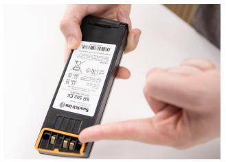
**2.1** Check before use that the gasket around the opening to the battery terminals are undamaged.
