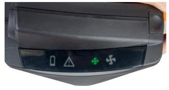
**8.3** If the flow meter outlet is now unblocked and the air is allowed to flow freely, the alarm signals will cease within 10 - 15 seconds.
