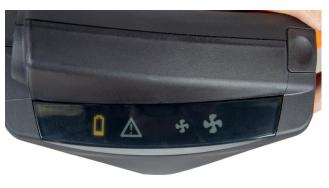
**6.5** If the battery capacity has dropped to about 5-10 % of the original charge, this is indicated as follows:
