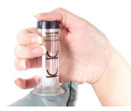
**8.1** Cause a flow stoppage by still holding tightly the joint between the hose and the flow meter bag and then blocking off the flow meter outlet.
