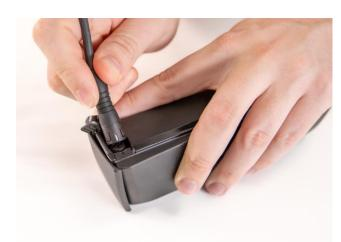
1.3 Connect the battery to the battery charger. Connect the charger plug to a wall socket.N.B. Main voltage 100-240 V
