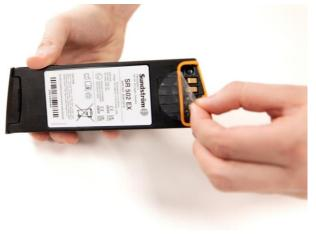
**1.2** Remove the tape and charge the battery.
