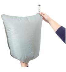
**7.3** Place the head top in the flow meter bag and start the fan.
