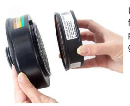
**10.4** To change the gas filter: Unscrew the filter/combined filter. To change the gas filter, prise the particle filter off the gas filter. Both filters/combined filters must be changed at the same time and must be of the same type and class.
