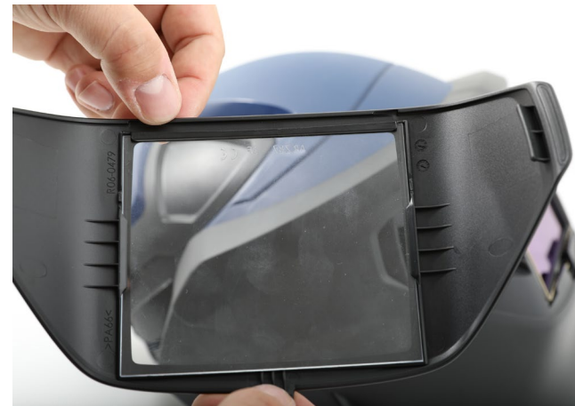
3.4 Control that the protective lens is mounted correctly.
