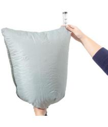
**2.3** Place the head top in the flow meter bag and start the fan unit.
