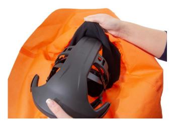
**1.2** Fit the head harness and air-duct into the hood.
