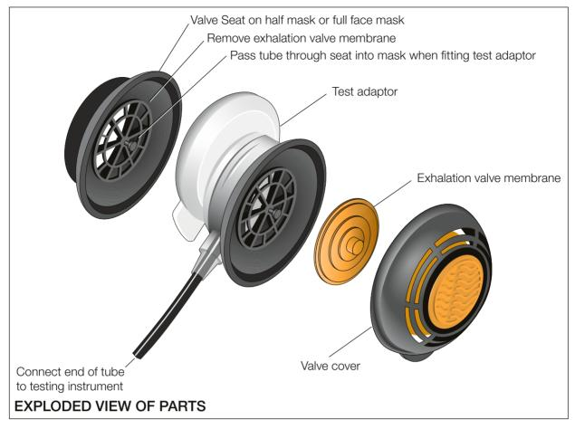
The SR 328 Test Adaptor is used to connect the half mask or full face mask to a measuring instrument for facial fit testing. The adaptor is fitted to an exhalation valve of the half mask or full face mask.
