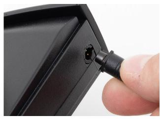
**2.1** Connect the battery to the battery charger.
