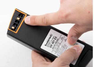
**3.1** Check that the gasket around the opening to the battery terminals on the underside of the battery is undamaged.
