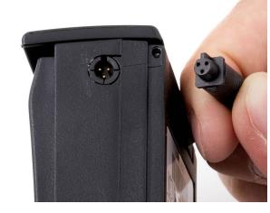
**2.2** Make sure that the pin on the cord's plug is fitted into the groove on the battery.
