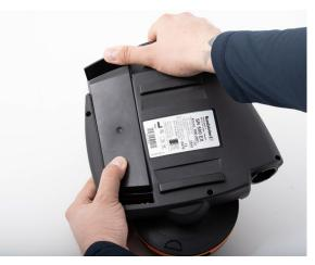
**1.2** Raise the battery cover a few centimeters and push with the thumb and withdraw the battery.
