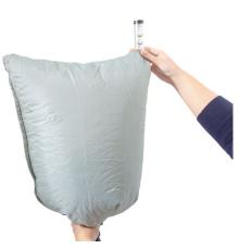
9.3 Place the head top in the flow meter bag and start the fan.
