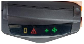
**6.2** After the button has been pressed, a programmed test will be run on the fan and the display will then light up, the audible signal will sound.
