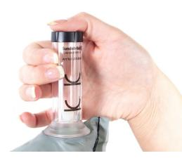
**10.1** Cause a flow stoppage by still holding tightly the joint between the hose and the flow meter bag and then blocking off the flow meter outlet.
