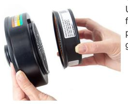
**12.4** To change the gas filter: Unscrew the filter/combined filter. To change the gas filter, prise the particle filter off the gas filter. Both filters/combined filters must be changed at the same time and must be of the same type and class.
