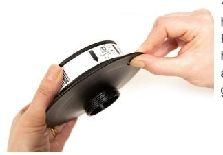
**12.2** Grip the filter with one hand. Place the thumb of the other hand on the underside of the adapter at the semicircular gap. Then prise out the filter.
