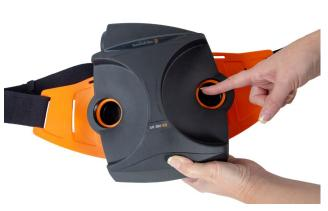
**5.3** Check that the gaskets in the filter mounting of the fan unit are in place and are in good condition.
