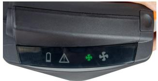
**6.3** After the internal test, all symbols will be extinguished except the small green fan symbol. This indicates normal operating status with a flow of at least 175 I / min.
