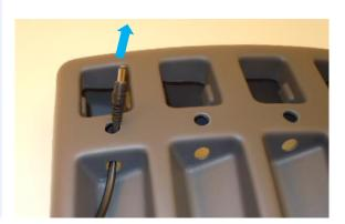
Connect the cable B to battery charger. Place excess cable inside the charging station & place battery charger in the designated compartment
