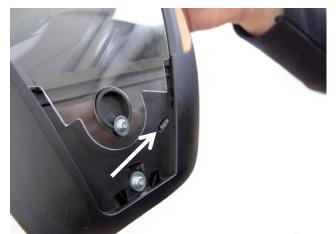
**5.4** Press the face seal frame down so that the pins drop into the visor unit holes. A clicking sound indicates that they are in place.
