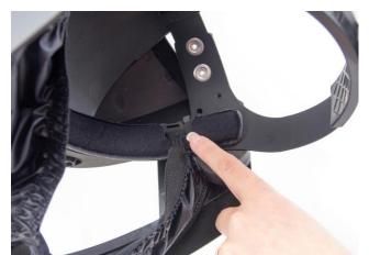
**6.4** Secure the hooks to the head harness where a relief has been made in the sweatband.
