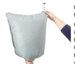
**2.3** Place the face shield in the flow meter bag and start the fan.
