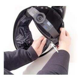
**5.2** Release the face seal by pulling it's frame so that its pins are released from the visor unit holes.
