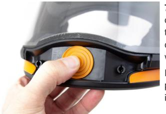
**7.4** Press the new membrane onto the pin. Carefully check that the membrane is in contact with the valve seat all way round.
