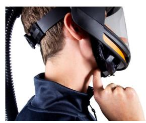
3.5 Insert a finger between your chin and the face seal and run the finger along the contact surface of the face seal all the way round to check that it fits well against the face.
