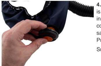
**4.1** The exhalation membrane is mounted on a pin on the inside of the valve cover. The cover must be changed at the same time as the membrane. Proceed as follows:
