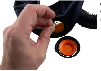
**6.4** Remove the membrane. Clean the exhalation membrane
