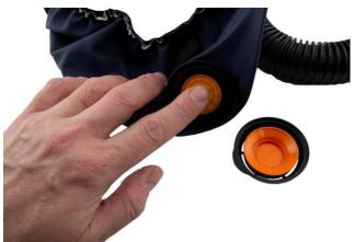
**4.3** Press the new membrane onto the pin. Carefully check that the membrane is in contact with the valve seat all way round.
