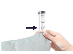
2.2 Place the head-top in the flow meter and start the fan unit. Grip the bag to seal around the breathing hose.Grip the flow meter tube with the other hand, the tube will point upwards from the bag
