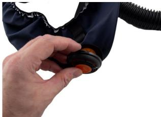
**6.3** Snap off the valve cover from the valve seat.
