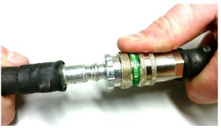
Carefully separate the nipple and coupling to prevent eventual air chock if there is pressure in the hose/system.
