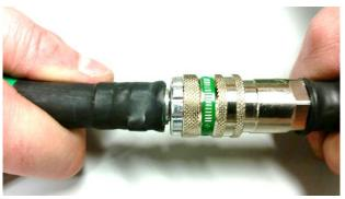
The locking ring then moves forward when it get into locked position.
