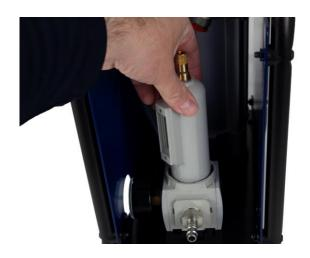
3.2 Remove the drain bowl Press it downward and twist anti-clockwise (bayonet mounting). Wash the bowl in hot water (not solvent) at a maximum of 140 F (60°C).
