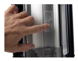
1.4 The filter element is fitted prior to delivery. Note the date on the label at the outside of the filter housing to be enable you to keep track of the date when the filter should be changed.
