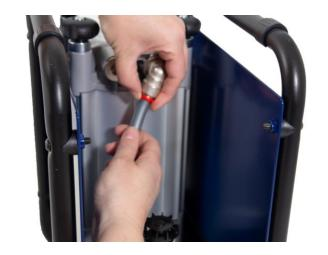
2.2 Loosen the hose between the regulator and filter lid by pushing the red sleeve on the coupling and disconnect the hose from the lid.
