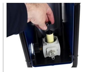
**3.3** Remove the pre-collector element by turning it anticlockwise.
