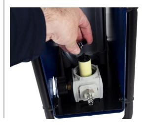
**4.3** Blow the parts clean with compressed air. Check that the drain outlet is not obstructed.
