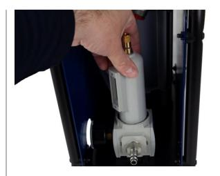
**4.2** Remove the drain bowl. Press it downward and twist anti-clockwise (bayonet mounting). Wash the bowl in hot water (not solvent) at a maximum of 140 F (60°C).
