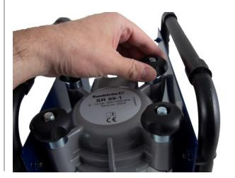
**2.3** Unscrew the knobs of the filter housing and remove the lid.
