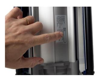
1.4 The filter element is fitted prior to delivery. Note the date on the label at the outside of the filter housing to be enable you to keep track of the date when the filter should be changed.
