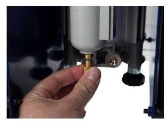
1.3 The filter is automatically drained to the given level. The drain can also be opened manually by turning the precollector at the bottom of the drain bowl.
