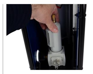
**4.2** Remove the drain bowl. Press it downward and twist anti-clockwise (bayonet mounting). Wash the bowl in hot water (not solvent) at a maximum of 60 °C.
