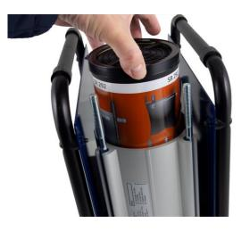
**2.4** Remove the used filter element.
