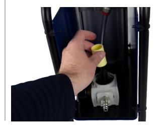
**3.4** Blow the parts clean with compressed air. Check that the drain outlet is not obstructed.
