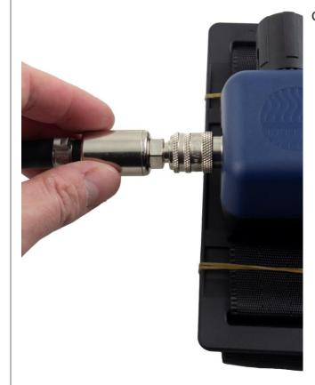
**6.2** Connect the breathing hose to the control valve outlet.
