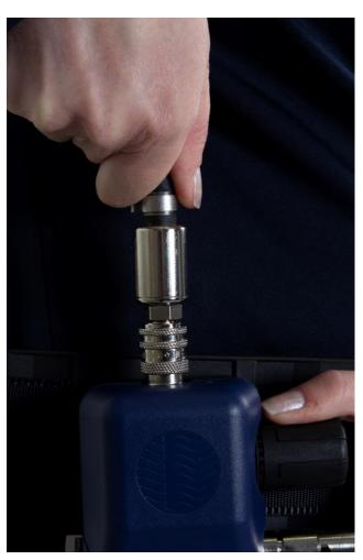
**9.1** Both couplings are of safety type and are released in two stages.
