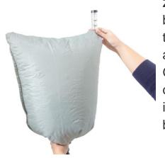
2.4 Place the facepiece in the bag and grip the opening of the bag so that it seals around the breathing hose. Grip the flow meter with the other hand and hold it so that it points vertically up from the bag.
