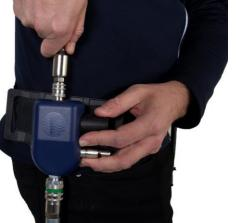
**8.2** Disconnect the compressed air hose from the control valve.
