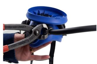
**12.2** Thread the hose clip and retaining clip onto the new hose. Connect to the mask and use a pair of pincers to nip the hose clip.
