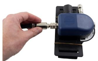
2.1 Check that the air flow measured through the mask is at least 150 l/min.
