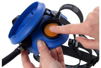
10.3 Press the new membranes onto the dowels.Carefully check that the membranes are in contact with the valve seats all round.
