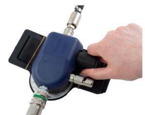
2.3 Turn the control valve knob anti-clockwise as far as it will go, in order to throttle the air flow rate to a minimum.
