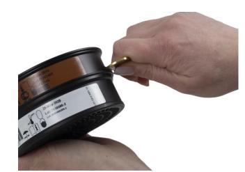
3.4 To separate a combined filter, place a coin it in the space between the lower lip of the particle filter and the small tab molded into the side of the gas filter. Push firmly and twist the coin until the filter pops off.
