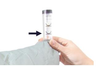
**2.2** Read the position of the ball in the tube. It should float level with or just above the marking on the tube 5.3 CFM (150 l/min).
