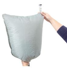
**2.1** Place the facepiece in the bag and grip the opening of the bag so that it seals around the breathing hose. Grip the flow meter with the other hand and hold it so that it points vertically up from the bag.
