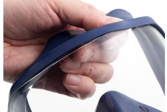
**12.5** Carefully prise the top half of the face piece over the visor and make sure that the visor is in the groove in the mask.
