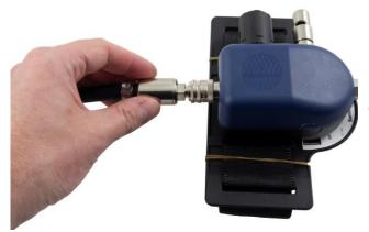
**1.4** Check that the air flow measured through the mask is at least 5.3 CFM (150 l/min) Connect the breathing hose of the mask to the control valve.
