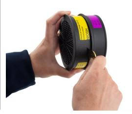
**3.4** Place a coin it in the space between the lower lip of the particulate filter and the small tab moulded into the side of the gas filter. Push firmly and twist the coin until the filter pops off.
