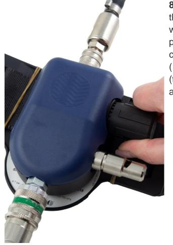
**8.1** Use the control valve knob to set the air flow rate to suit your current work intensity. In the fully closed position (turn the knob anticlockwise), the flow is about 5.3 CFM (150 l/min). In the fully open position (turn the knob clockwise), the flow is about 13.8 CFM (390 l/min).
