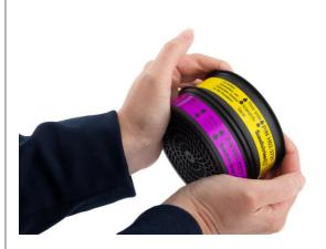
**3.3** Place the particulate filter on top of the cartridge. Grasp both protective elements. Squeeze hard until you hear the particle filter snap onto the gas filter.
