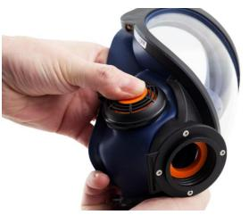
**14.4** Press the valve covers into place. A clicking sound indicates that the cover has snapped into place. Carry out a negative fit check.
