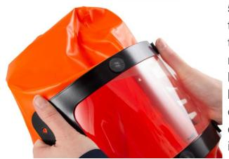
5.8 Press the visor towards the frame all round, so that the tape will stick to the hood material. Fit the head harness. Make sure that the beads in the mounting plate of the head harness are oriented into the guide holes in the visor.
