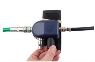
**1.2** Connect the compressed air supply tube to the control valve.
