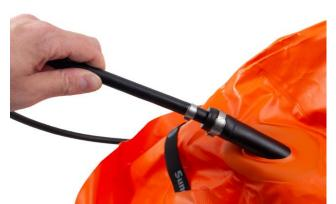
**6.4** By pulling the hose, check that it is firmly secured to the hood.
