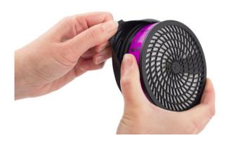
2.1 Fit the filter/combined filter in the filter adapter so that the arrows on the filter point towards the user's face. Carefully check that the edge of the filter is in the internal groove of the filter mounting all around.
