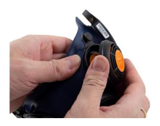
**8.1** The exhalation membranes are mounted on a fixed dowel on the inside of the valve covers on each side of the outer mask. The covers should be changed whenever the membranes are changed. Snap the valve covers off the valve seats.
