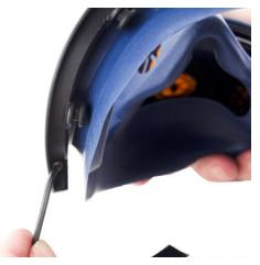
6.1 The visor is mounted in a groove running around the visor opening of the outer mask and is held in place by one upper and one lower frame half. Use a 2.5 mm Allen key to remove the two screws holding the frame halves together.
