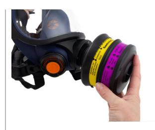
2.3 Turn the filters into the mask. Screw until the thread reaches the seal at the bottom of the filter connection, then another 45 degrees.
