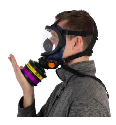
**5.1** Place the pre-filter holder to the filter. Put the mask on. Place the palm of your hand lightly over the hole on the pre-filter holder to make it tight. NOTE! Do not push so hard that the respirator's shape is affected. Take a deep breath and hold your breath for about 10 s. If the mask is tight, it will be pressed against your face. If any leakage is detected, check the inhalation and exhalation valves or adjust the straps of head harness. Repeat the fit check until there is no leakage.
