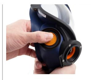
8.3 Press the new membranes onto the dowels.Carefully check that the membranes are in contact with the valve seats all round.
