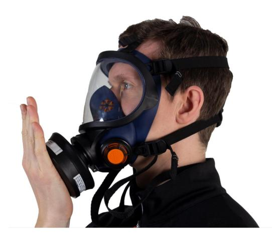
**5.1** Place the pre-filter holder to the filter. Put the mask on. Place the palm of your hand lightly over the hole on the pre-filter holder to make it tight. NOTE! Do not push so hard that the respirator's shape is affected. Take a deep breath and hold your breath for about 10 s. If the mask is tight, it will be pressed against your face. If any leakage is detected, check the inhalation and exhalation valves or adjust the straps of head harness. Repeat the fit check until there is no leakage.
