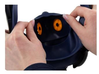
**7.2** Two membranes are fitted, i.e. one on each inside of the inner mask. The dowels for these membranes are removable and should be changed whenever the membrane is changed. Prise off the membranes and dowels.
