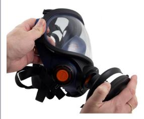
**2.3** Turn the filters into the mask. Screw until the thread reaches the seal at the bottom of the filter connection, then another 45 degrees.
