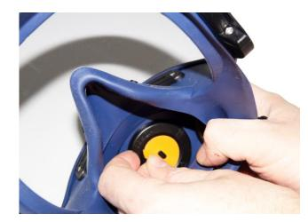
**7.1** One membrane is in the center of the inner mask on a fixed dowel. Prise off the membrane and fit a new membrane.
