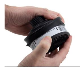
**2.1** Fit the filter/combined filter in the filter adapter so that the arrows on the filter point towards the user's face. Carefully check that the edge of the filter is in the internal groove of the filter mounting all around.
