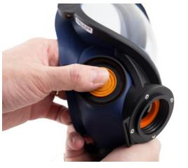
**8.3** Press the new membranes onto the dowels. Carefully check that the membranes are in contact with the valve seats all round.
