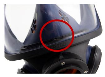
**6.4** Markings are made to show the centers of the visor, frame halves and mask. Press the new visor into the groove, making sure that the center markings are in line. To make assembly easier, coat the slot with a soap solution or similar liquid.
