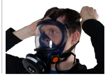
**4.4** Tension the elastic straps in pairs by pulling the free strap ends towards the rear. Adjust the fit of the mask on your face, so that it fits firmly but comfortably. Adjust the lengths of the upper pair of straps and fix by means of the buckles.
