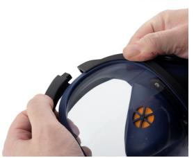
**6.2** Carefully remove the upper frame half. Carefully prise the top part of the mask off the visor and remove the visor from the lower groove.
