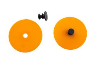
**7.3** Prise the new membranes onto the new dowels. The membrane should rest on the larger flange, i.e. thread the dowel with the membrane from the inside of the mask, through the valve seat, with the smaller flange first.
